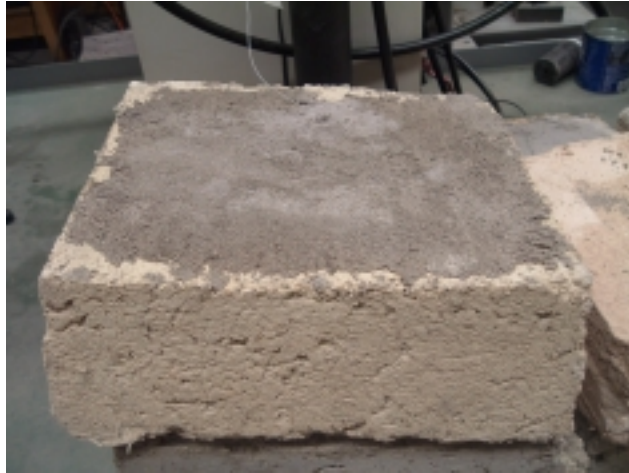
Figure 1.- Papercrete sample with mortar on one face
